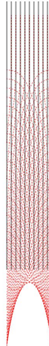
Fig. 14b: Asymptotic curves merge into facade
