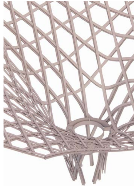
Fig. 10: Axonometric of typical support, metal ring fixing the place of the timber
