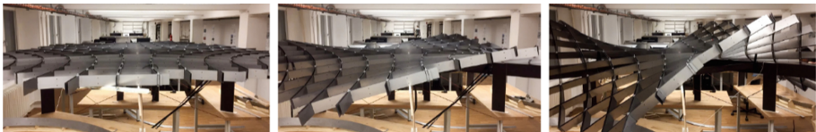
Fig. 2. Kinetic behaviour of the first asymptotic steel grid. The lamellas are assembled flat and transform into the design shape simply by a push of the hand. They are constrained by the strong axis of lamellas and the scissor joints.
